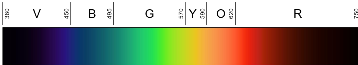
Figure 4—The spectrum of visible light. The numbers give the wavelength in nm. The letters refer to the colors: Violet, Blue, Green, Yellow, Orange, and Red.
